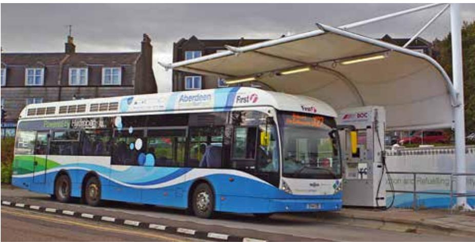
The site has the capacity to produce 360kg of hydrogen daily. That is enough for the current fleet of 10 x 42-seat buses to travel up to 350km each day emitting nothing more than clean water produced from the tail pipes.
